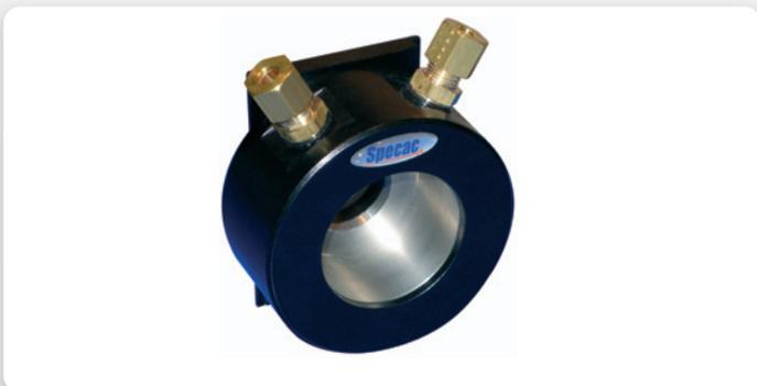
The Water Heating Jacket is similar to the Electrical Heating Jacket, but it uses circulating water to heat the sample cell. A jacket around the circular aperture is filled with a solution, for example water, heated by a thermocirculating system. Temperature control of the sample holder is reliant upon this thermocirculating system.
