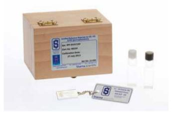
To allow users flexibility in use the reference is supplied with certified wavelength and absorbance values at two different bandwidths, 1.0 nm and 5.0 nm. Nominal values are given below.
