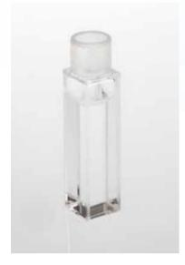
10 mm far UV quartz fluorometer cuvette with polished faces at 90° containing ultra-high purity water, permanently sealed by heat fusion.
