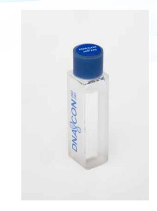
Absorbance values are certified at 260 nm, 280 nm and 330 nm at spectral bandwidths of 1.0, 2.0, 3.0, 4.0 and 5.0 nm. The value at 330 nm is used as a "background" correction, as in the normal methodology. From these values a corrected 260/280 ratio is calculated for each bandwidth using the formula:
