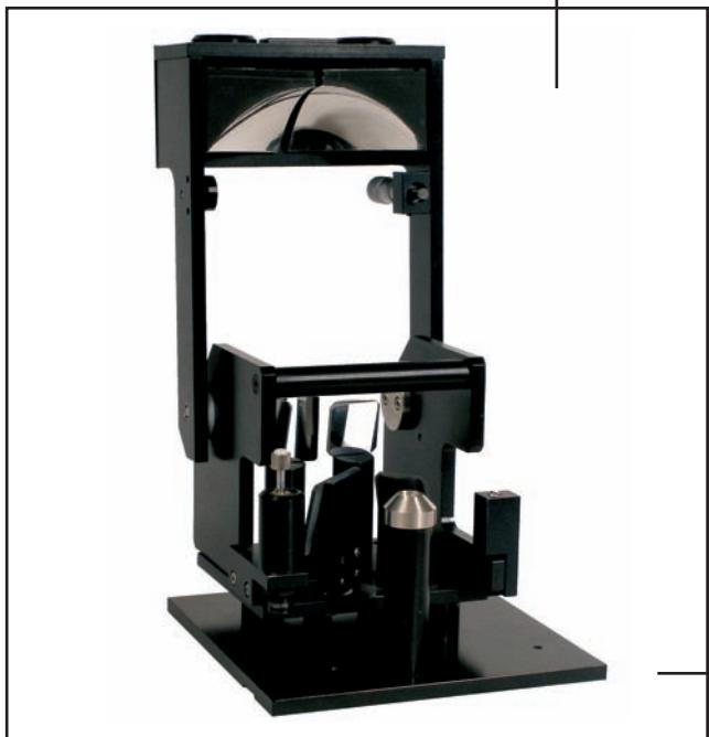
**Diffuse reflectance is based upon the collection of radiation that has been diffusely scattered from the sample. The Specac Selector uses an optimized off-axis optics configuration which selectively collects the diffusely reflected components, whilst minimizing the specular component.**
